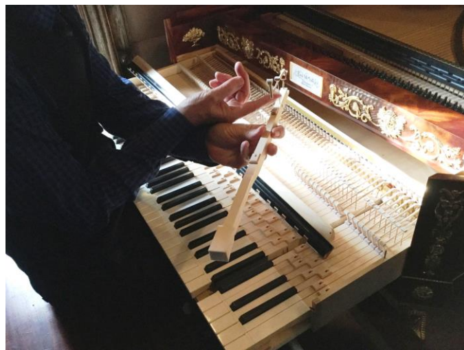
The action inside a replica 1810 forte piano, built in the Czech Republic in 2017
